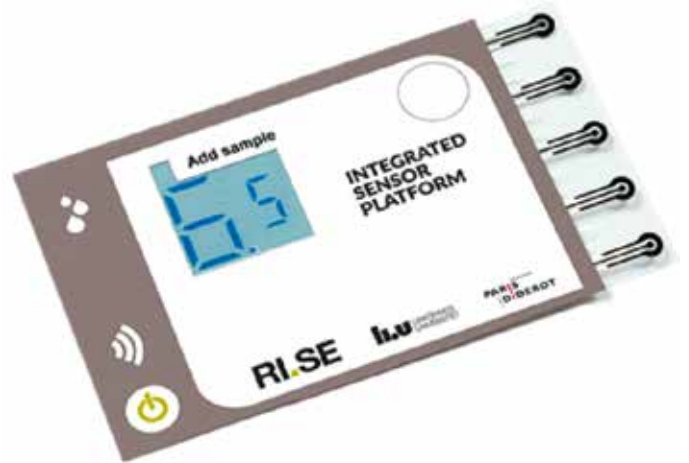
Integrated printed biosensor platform by RISE Acreo, leader of GREENSENSE's WP4 - printing and curing of functional inks on NC and WP5 - printed electronic components development with NC
