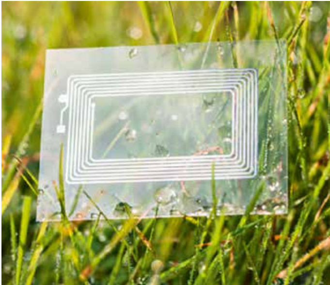
RFID antenna printed with Ag nanoink by Genes'Ink, leader of GREENSENSE's WP3 - NC based inks formulation
